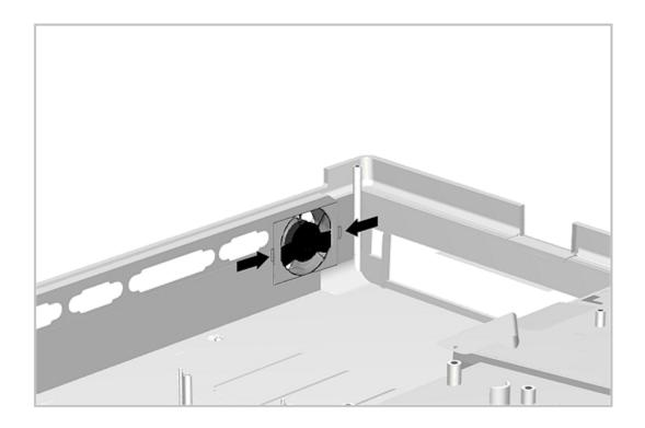
Figure 7-21. Removing the Auxiliary Fan
